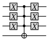
$$\begin{array}{c|c} |x_1\rangle \\ \hline U_0 \\ |x_n\rangle \\ |y\rangle \end{array} \begin{array}{c} |x_1\rangle \\ |x_n\rangle \\ |x_n\rangle \\ |y \oplus [x = 0...0]\rangle \end{array}$$
