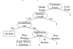
Figure 6: The top of the decision tree model built automatically by iComment trainer from Linux's lock-related comments.
