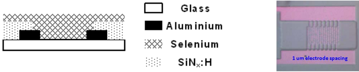
Figure 1. Cross-sectional diagram of fabricated lateral detector (left) and micrograph of the fabricated detector (right).
