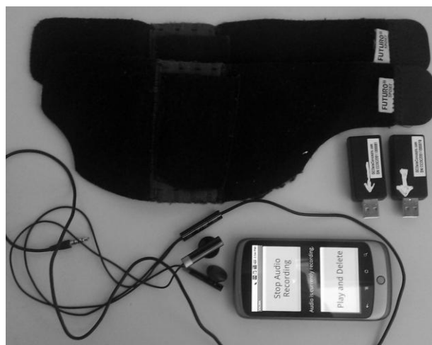
Figure 1: VALMA system components. Google Nexus One smartphone, headset, accelerometers and ankle straps.
